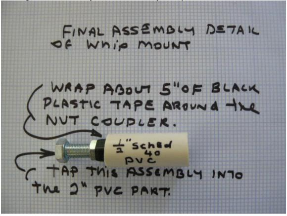
Now choose the last PVC adapter. It is the  $\frac{1}{2}$  inch slip to  $\frac{3}{4}$  inch slip adapter. Tap the nut coupler piece into the  $\frac{1}{2}$  inch slip side of that adapter.
