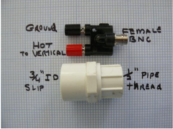
By attaching the above black and red connector to the PVC part pictured above, you will have a very easy way to connect the coax to the bottom of the fixture ( a BNC connection ) and it will make it easy for you to wire the antenna. See the assembly when it is finished:
