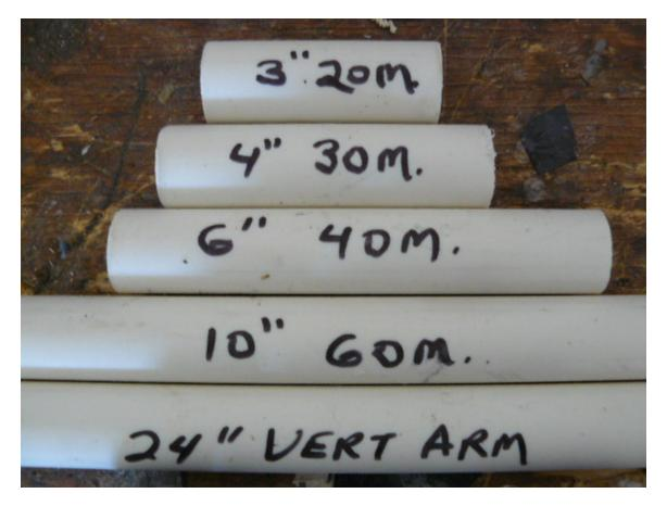
On each of the above forms, drill a 1/8 inch hole <u>all the way through</u> <u>the pipe</u> exactly an inch from each end. This will hold the wire to the coil forms.
