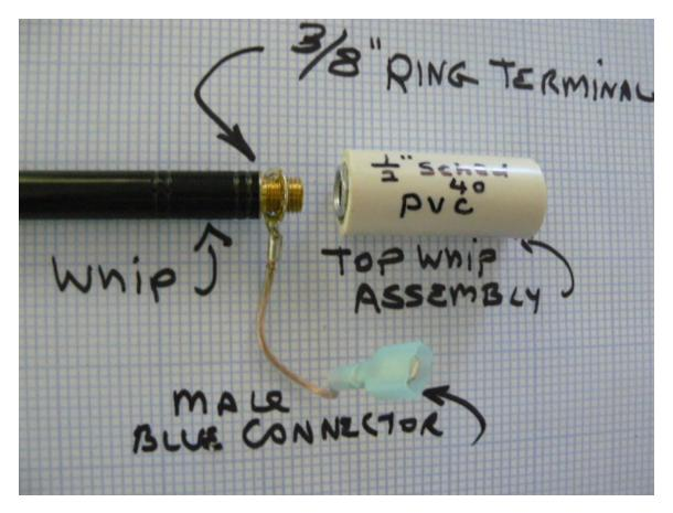
If you couldn't locate a ring connector, just make a loop in the wire with a big enough hole to accommodate the threaded whip until you can get the correct size of ring connector. The ring connector makes the connection much better strength-wise.
